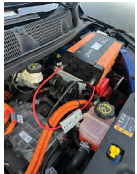
Chevy Bolt motor with inverter to power house appliances.
